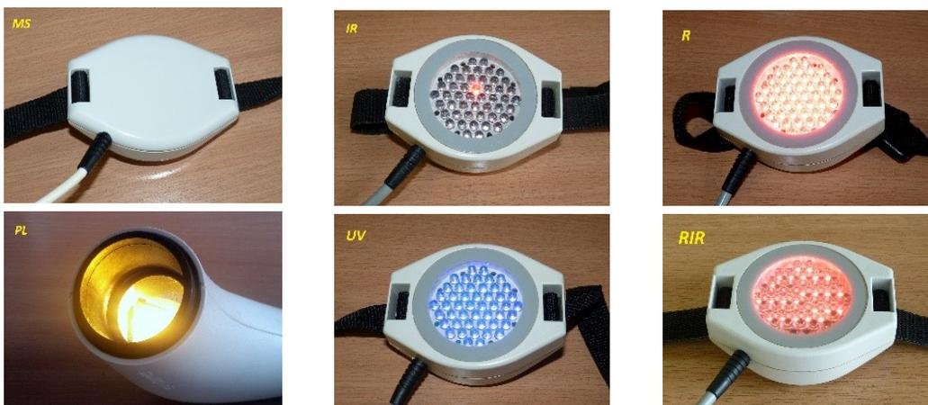
**Fig. 1. The elliptical applicator and magnetic-field+light applicators used in this study**
